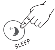
5 Press <SLEEP> button for 5s to renew program, and stop flashing <RESET>
